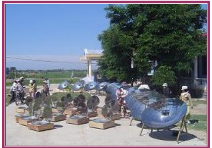
Cooking in the sun with parabolic and box cookers
