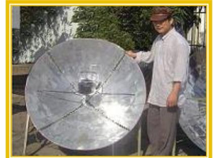
It took him some time, but he came up with the cooker you see in the picture. He used some cheap reflecting material for this first trial. Some other workers designed a foldable stand and together the result was almost similar to the normal parabolic cookers. We were very happy that this new parabolic cooker was working well. Now we must learn how to make the four part parabolic cooker faster. It will be a good model for export and also easy for local transport.
